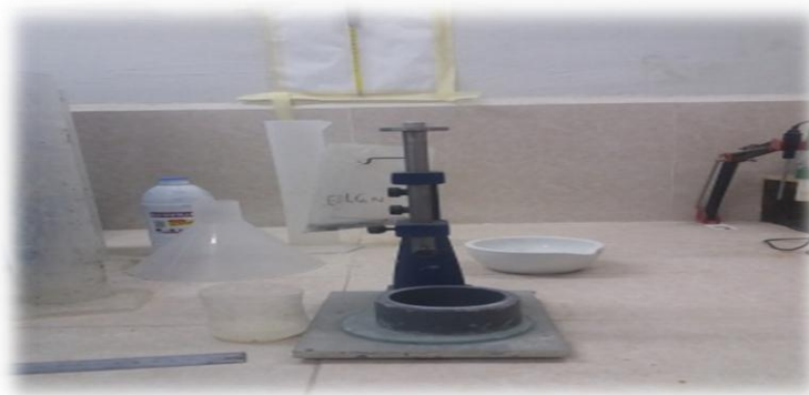
| Figure -24- appareil Vicat.
