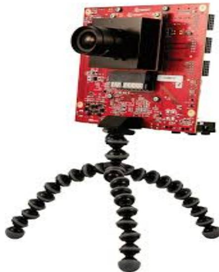
**Figure III.6 : Kit Caméra PYTHON-1300C-MicroZed Embedded Vision Carrier Card .**
