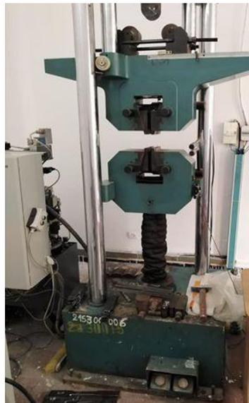
FigureII.11 : Machine de traction ZWICK/ROELL.
