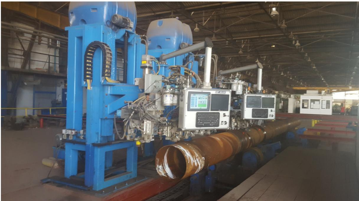
**Fig. 4.10 machine ultrason**
