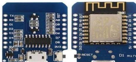
**Figure II.5:** Module shield wifi.
