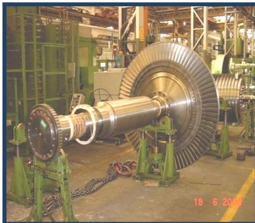
**Fig. I.11 :** Turbine haute pression HP
