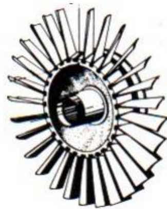
Figure 1-6 showing compressor rotor disk.
