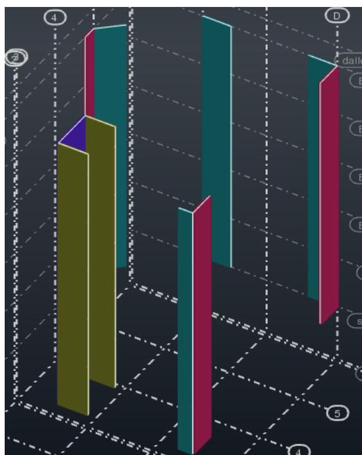
FIGURE 5. 6: DISPOSITION DES VOILES
