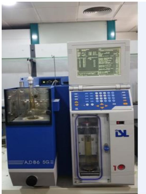
**Appareillage de distillation ASTM D86.**
