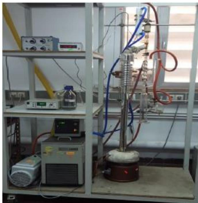
**Appareillage de distillation TBP manuelle ASTM 2892.**
