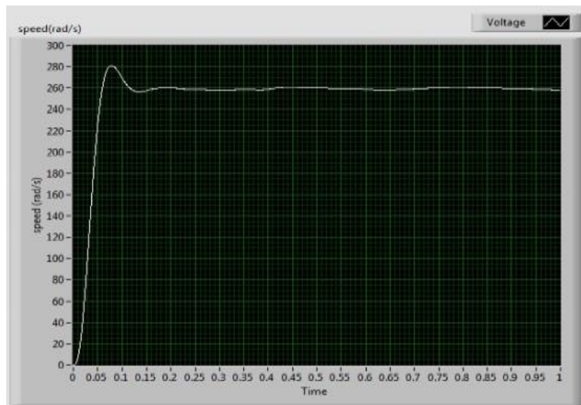
Figure 5.16: The speed of the DC motor for an input voltage of 12V.
