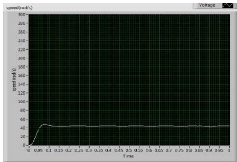
Figure 5.18: The speed of the DC motor for an input voltage of 3V.
