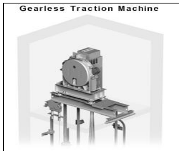
Figure 1.2: Configuration of Gearless traction lift
