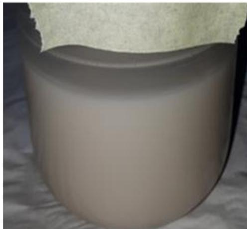
**Figure IV. 3 : suspension  $20 \text{ Kg/m}^3$  BC + 30% Chaux.**
