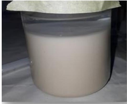
*La figure IV.6 : suspension 30 Kg/m<sup>3</sup>BC + 30% Chaux*
