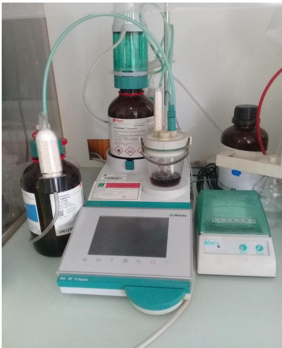
**Figure 5 :** Appareillage de Karl Fisher type (Metrohm)
