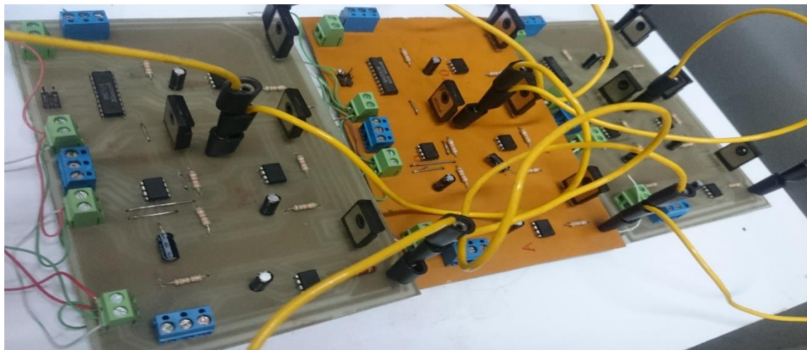
Figure 4.27 The T-type inverter designed in a PCB.
