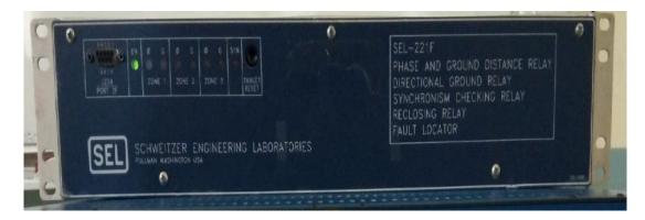
Figure 2.1: SEL-221F Numerical Distance Relay
