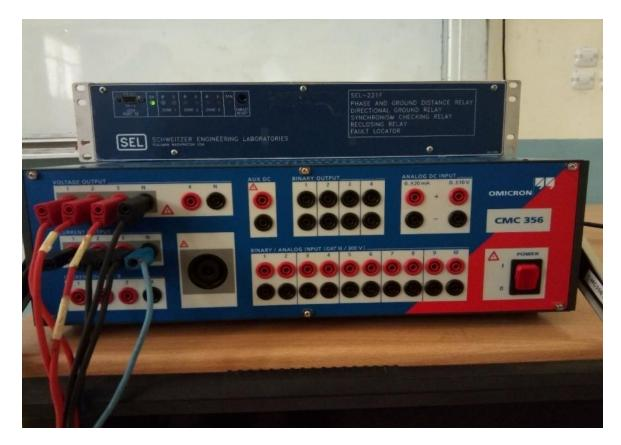
Figure 2.8: Front View of CMC 356 With Voltage and Current Outputs Connected
