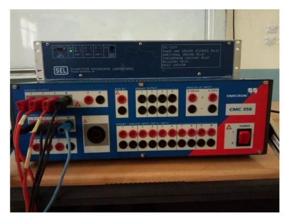
Figure 2.4: SEL 221 Relay and OMICRON CMC 356 Put Together In IGEE Lab Bench
