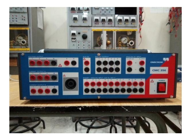
Figure 2.5: Injection Test Set OMICRON CMC 356
