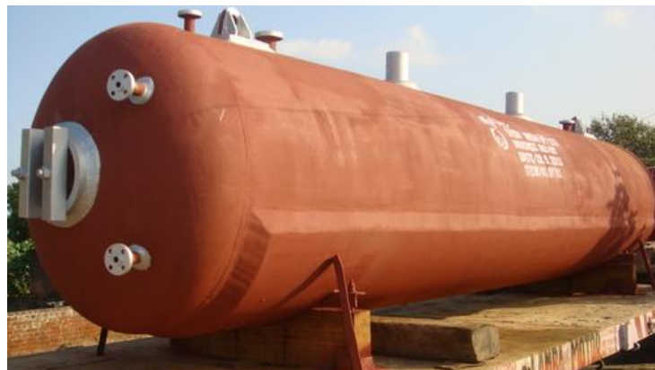
Figure 1.4 An Industrial Boiler Drum
