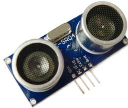
FIGURE 2.6 – Ultrasonic Sensor-HC-SR04
