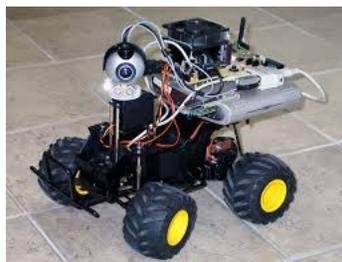
FIGURE 1.1 – Autonomous Mobile Robot
