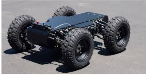
FIGURE 1.4 – Wheeled Robot
