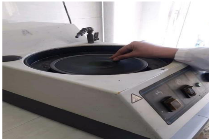
Figure II.10 : polissage de finition.
