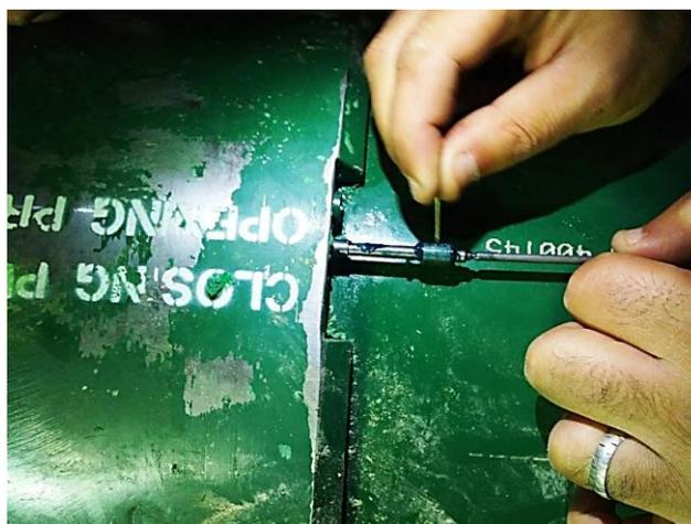
**Fig.21: Remove the existing shear pin and install the replacement shear pin (875psi)**
