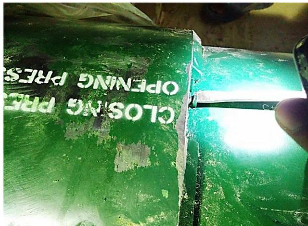
**Fig.24: Thread and tighten the valve retainer screw into the valve housing**
