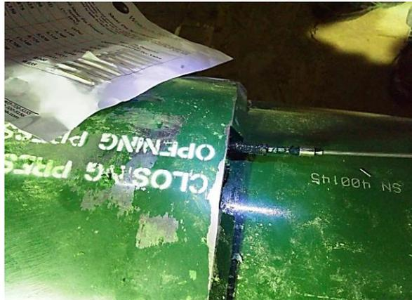
**Fig.17: Re-install the opening valve into the valve housing**
