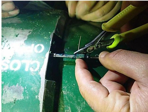
**Fig.22: Cut the replacement shear pin**
