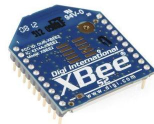
Figure IV. 22 Module XBee S2.[24]
