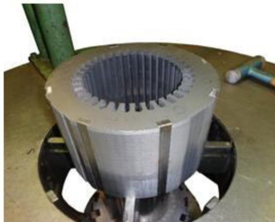
**Figure I. 5: Paquet statorique**
