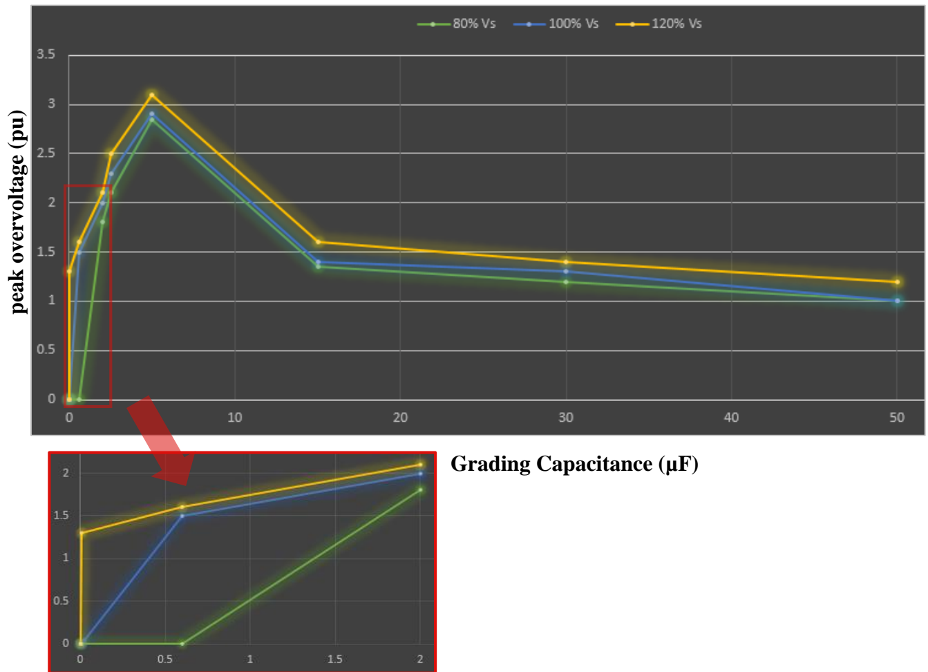
Figure 3.24: The effect of the grading Capacitance on ferroresonance.
