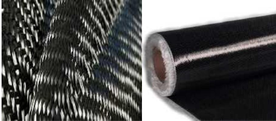
**Figure 1.8 :** fibre de carbone.
