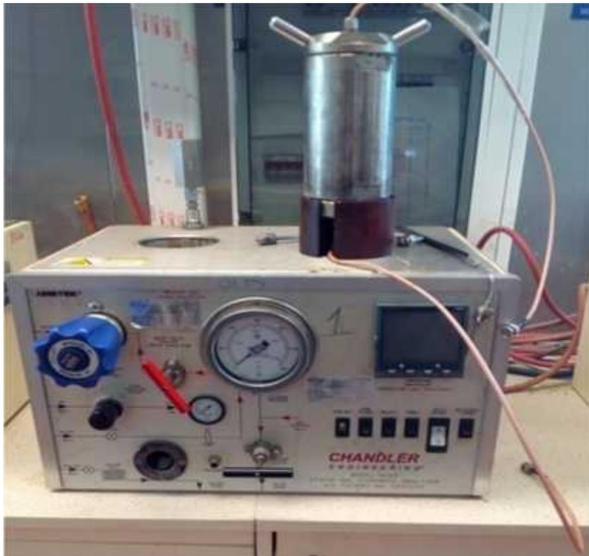
Figure (23): Static Gel Strength Analyzer (SGSA).
