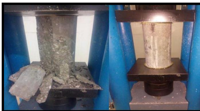
**Figure 22.** Essai de compression.
