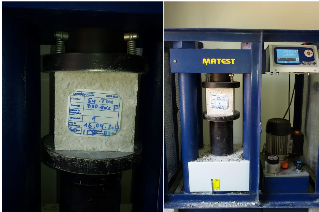
Figure III.10 : Essais de compression
