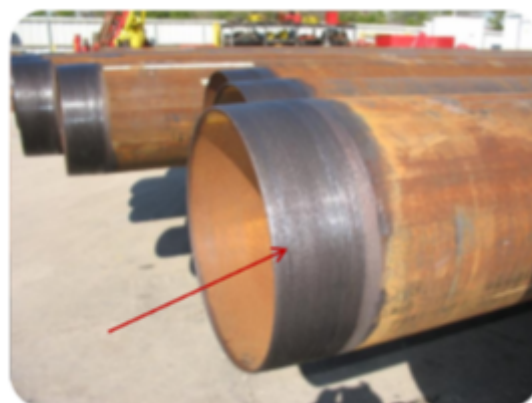
FIGURE 2.13 – Contrefort Pin with Pipe Dope Applied
