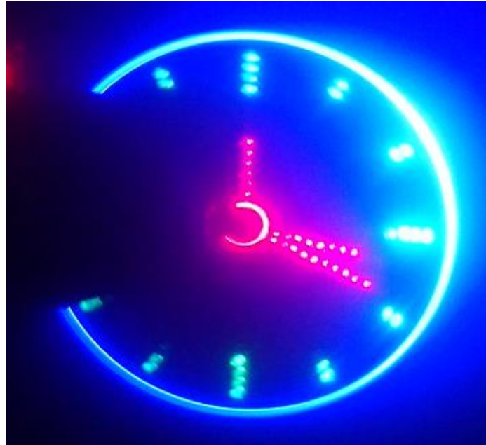
Figure 4.7. Propeller display of a clock that point to 12:16:19
