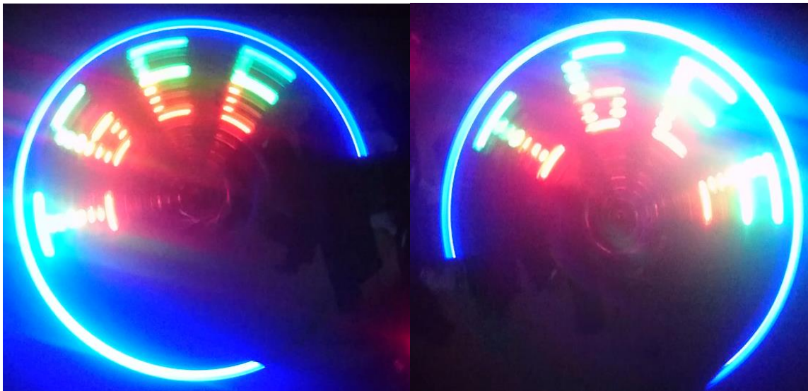
Figure 4.4. Propeller display of the string 'IGEE'
