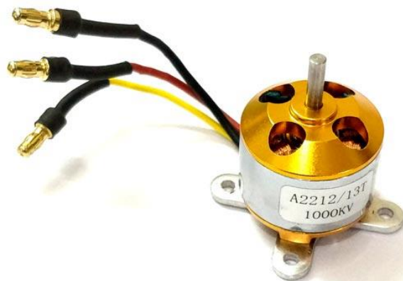
Figure 2.5. 2212 Brushless DC motor
