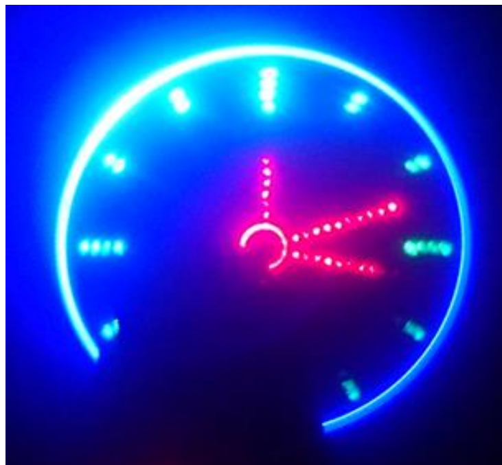
Figure 4.6 – Propeller display of a clock that point to 12:16:12
