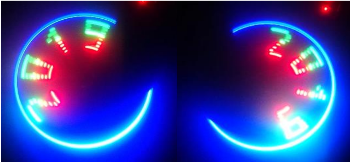
Figure 4.5. Propeller display of '2019'.
