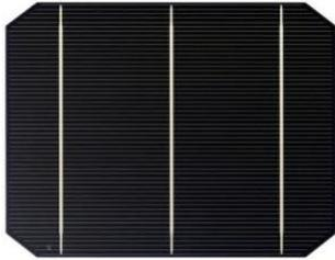
**Figure (I.2) :** cellule monocristalline.
