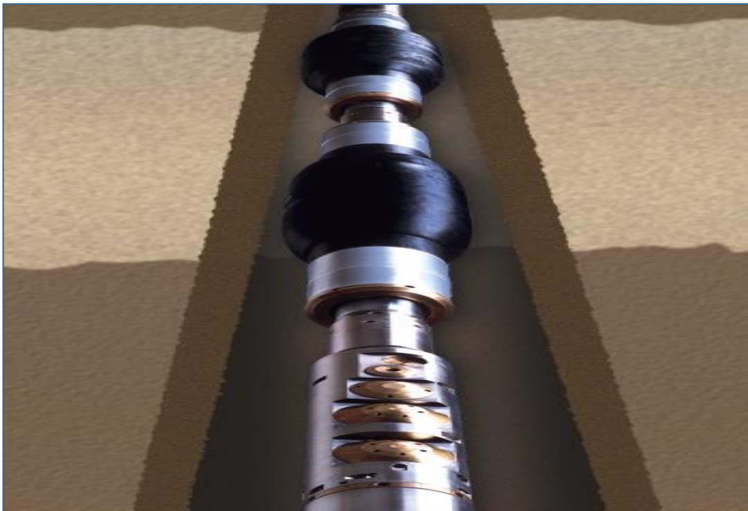
Fig.III.11: Module dual-packer (Schlumberger, 2002)
