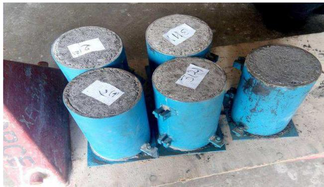
**Figure II.11:** Eprouvette Cylindrique (16×32 cm)
