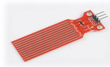
Figure I. 23 Water level sensor
