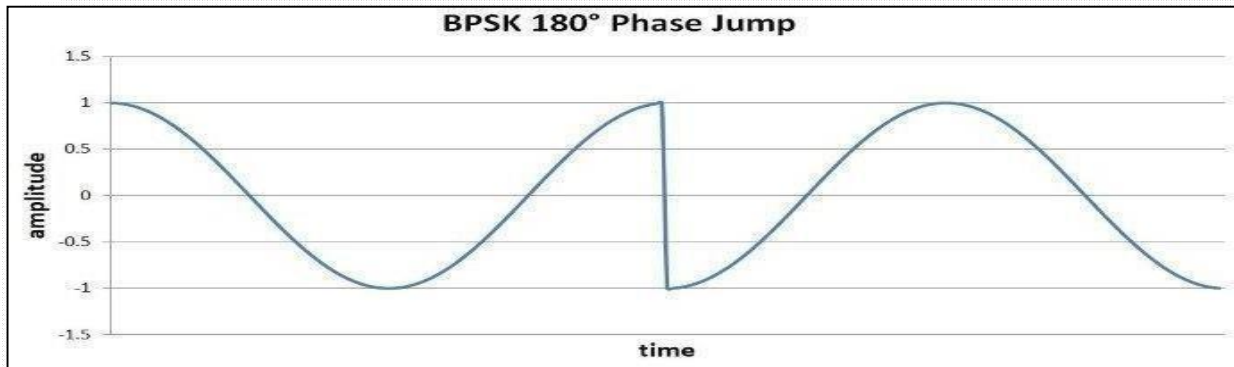
Figure II.5 BPSK 180° Phase jump[22]
