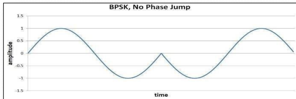
Figure II.6 BPSK, No Phase Jump [22]
