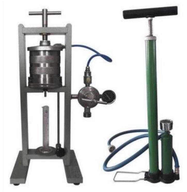
**Figure II.5** : Filtres-presses API
