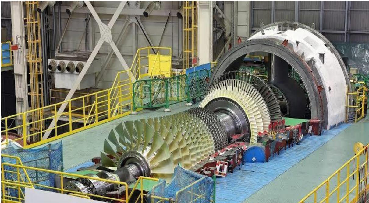
**Figure 8 : corps haute pression (HP)**
