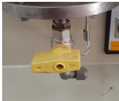
**Figure 3.8 :** La soupape de charge.
