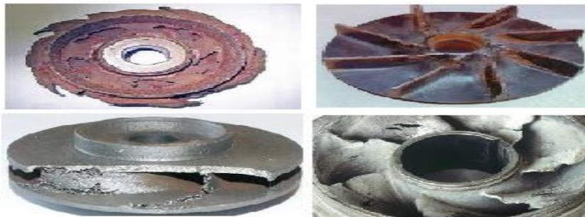
Figure I-11: Cavitation des pompes
