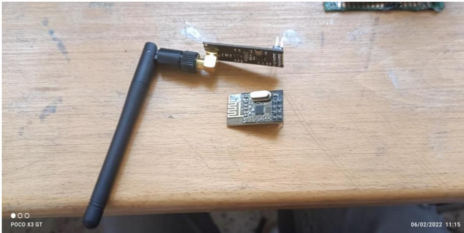
**Figure 3.7: Antenne radio NRF24L01 PA et NRF24L01**
