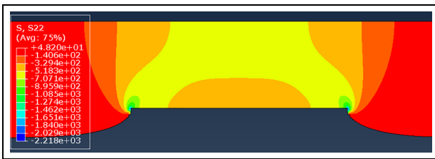
Figure 6. Contour of normal stress distribution on the layer thickness.
