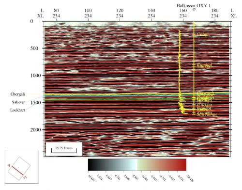
Figure 8. Interpreted seismic section of crossline 234 at the Balkassar OXY 01 well. Three horizons including the Chorgali Formation (yellow), Sakesar Limestone (blue), and Lockhart Formation (green) are marked on the seismic section. The well Balkassar OXY 01 along with formation picks is plotted on the section. The horizons show a flat trend, as the seismic cube only covers the central flat portion of the Balkassar box fold anticline.
