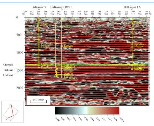
**Figure 9.** Interpreted arbitrary seismic line passing through all three wells of the study area. The line is selected to pass through all three wells used in the study to show the regional trend in the north—south direction. A gentle bulge is observed toward the Balkassar 07 well in the southern part of the study area. Formation picks of all drilled formations in three wells are shown in the figure with yellow color.
