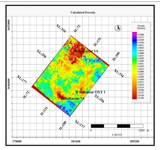
**Figure 14.** Porosity slice extracted from the computed porosity model at the top of the Sakesar Limestone. Predicted porosities using the PNN analysis show that the formation bears tight reservoir conditions throughout the study area. The northern part of the field represents extremely tight conditions with porosities less than 1%; however, the southern part of the study area exhibits a porosity range at 4-7%.
