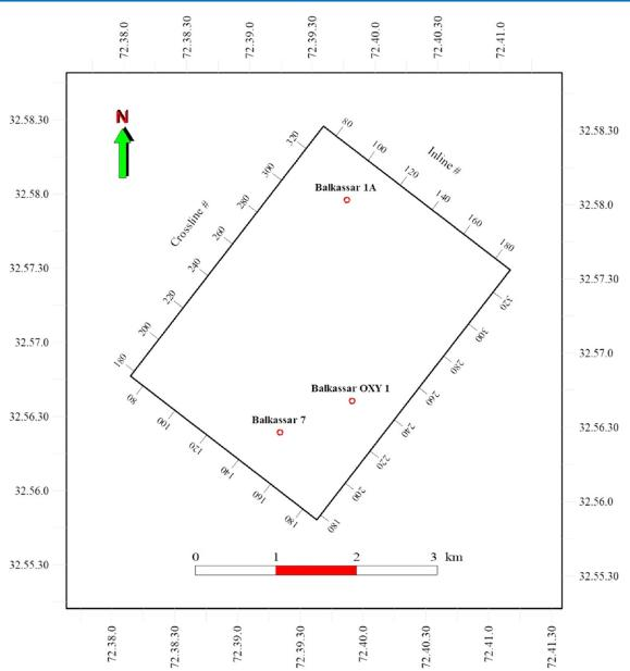
**Figure 3.** Base map of the Balkassar area showing the boundary of the 3D seismic cube and location of wells. Three wells including Balkassar OXY 01, Balkassar 07, and Balkassar 01 A along with a  $10 \text{ km}^2$  seismic cube covering the central part of the Balkassar anticline are utilized in this study. Crosslines are oriented in the northwest–southeast direction, and inlines are oriented in the northwest direction.
