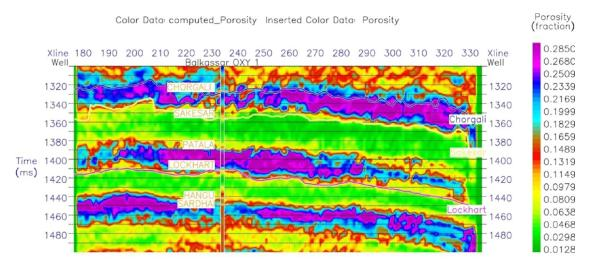
**Figure 13.** Computed porosity section of the study area through the Balkassar OXY 01 well using PNN. Predicted porosities in the Sakesar Limestone are less than 4% throughout the porosity section represented by the green color fill. This low porosity correlates with the porosity values computed from log data and validates the high impedance intervals.
