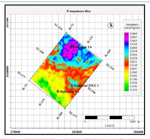
**Figure 12.** Inverted Zp slice extracted from the P-impedance model at the top of the Sakesar Limestone. The impedance slice of 20 ms averaging window is selected to display the lateral variations of impedance throughout the area with the help of color fills. The northern part of the area where the Balkassar 01A well is drilled represents a high-impedance zone (magenta color fill), whereas the southern part depicts low impedance values (green color fill).
