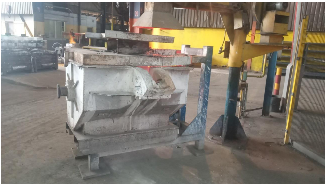
Figure 10: Poche de coulée
