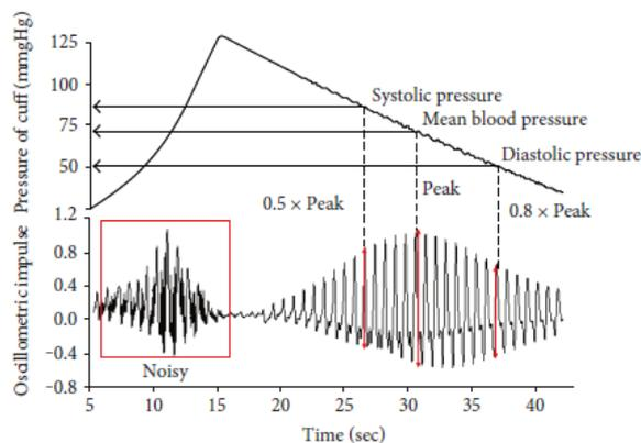
Figure 2 : SBP/DBP measurement technique in the Oscillometric method.
