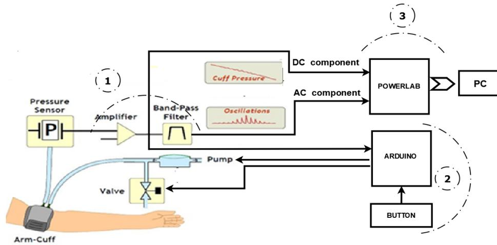
Figure 1: Diagram bloc of the oscillometric blood pressure measurement
