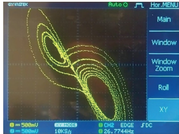
Fig. 9. The Lorenz Attractor XY on the oscilloscope
