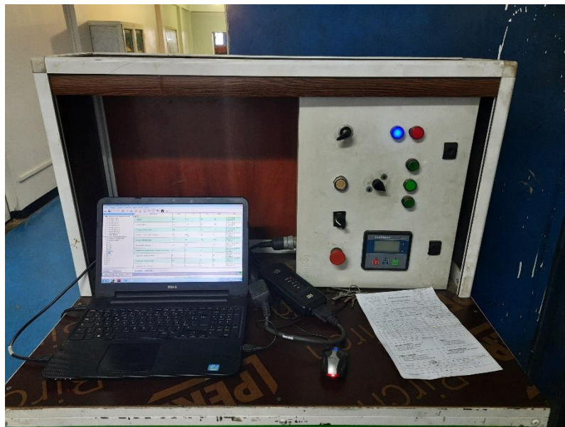
Figure III.06: Installation de l'adaptateur ComIII.
