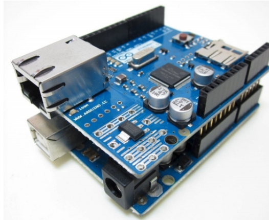
Figure 3.10: Ethernet shield W5100 plugged in an Arduino Uno board
