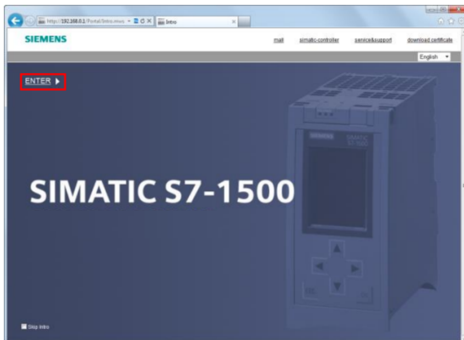
Figure 3.19: Example of S7-1500 Webpage interface
