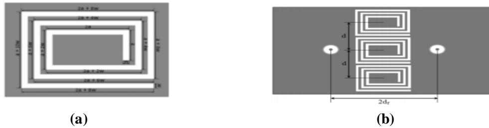
Figure 1.11: (a) Complementary split spiral Resonator, (b) The proposed microstrip antenna (CSSR) unit cell [16].
