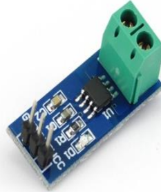
Figure 3.18 ACS712-05BT Hall Effect current sensor.
