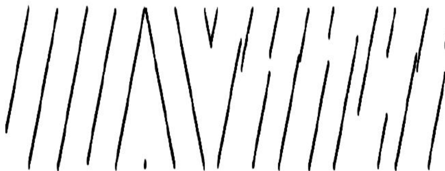
Figure 2.3: Spectrogram representation of LoRa Packet
