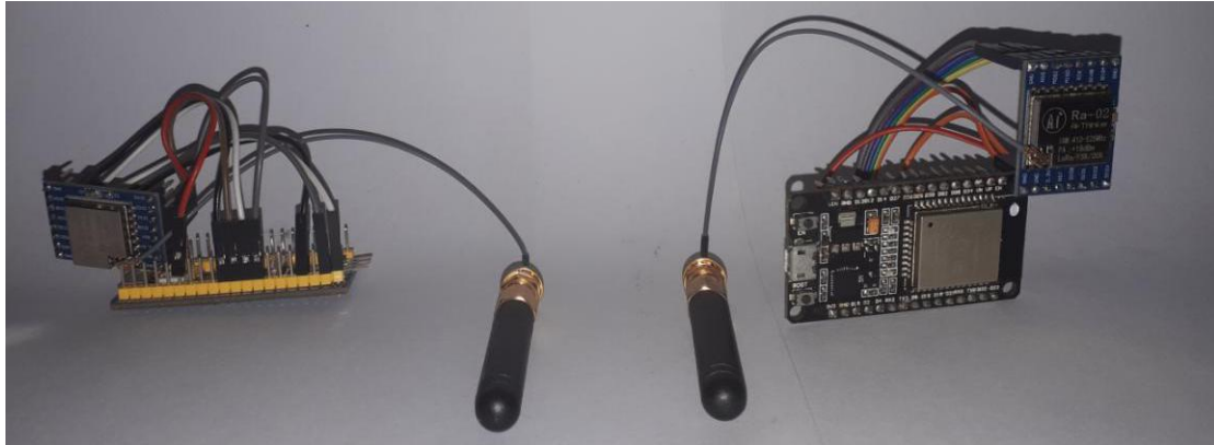
Figure 4.1: Node (left) to gateway (right) communication test (close-range)
