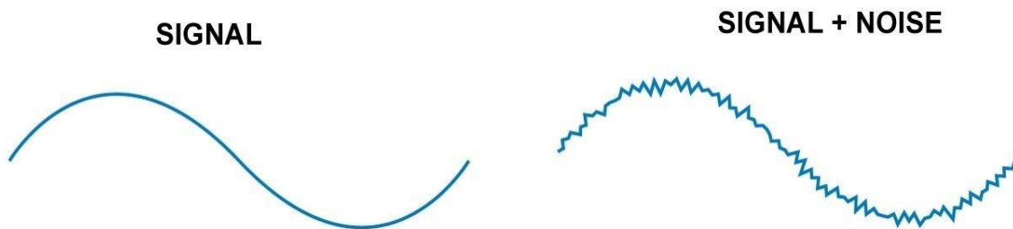
Fig.1.5 Waveform shape of a signal with and without noise
